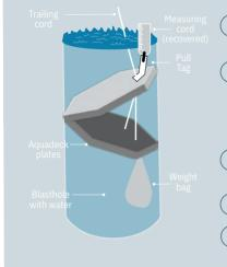
The Aquadeck uses a pair of geometrically proportional plates and unique mechanical system to create a deck in a blasthole regardless of the presence of water.
